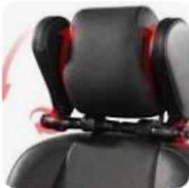
Head rests are optional passive equipment, but if the vehicle is equipped for safety reasons they must be used. During the sudden impact of the vehicle in the rear, the head moves backwards, in which case neck injury can also be caused. In order to avoid these injuries, head restraints are installed which must be suitable and provide good head support.
